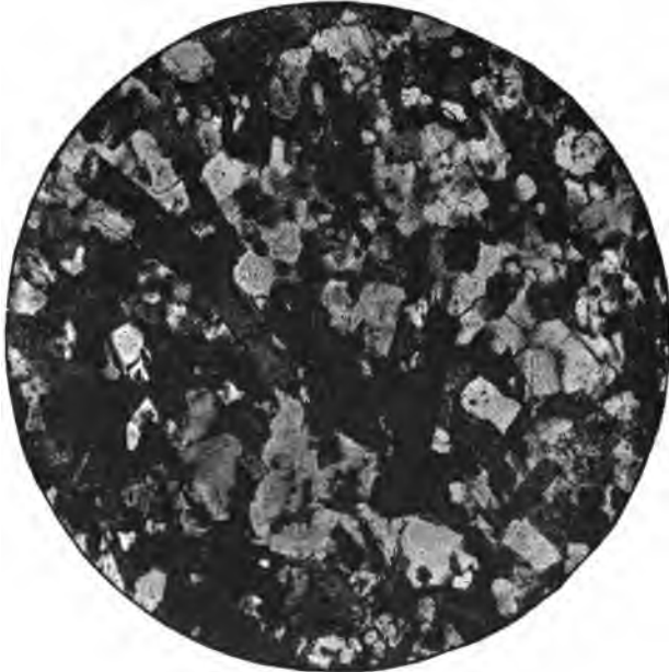
FIG. 2. — A thin section of mica schist, showing the crystalline structure which lends itself to the conversion of rock into soil.
